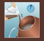
Pour this into the concrete / mortar and mix for 3-4 minutes. Discharge the concrete / mortar for application. Cure the applied concrete / mortar as per good construction practices
