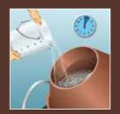
Add 3/4th of required water into the mixture and mix for 3-4 minutes
